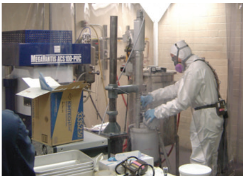
Figure 10. Nanomaterial worker wearing personal protective equipment in a work area with local engineering controls. Photo by Mark Methner, NIOSH.
