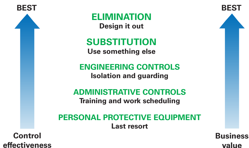
Figure 5. Hierarchy of Controls [adapted from ANSI/ASSE Z590.3 2011; AIHA 2008].
