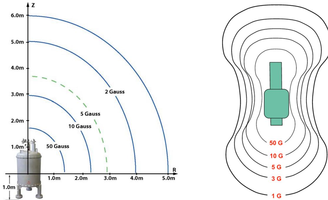
Based on the shape and orientation of the magnet, the resulting fringe field may not be circular; consult the manufacturer's specification sheet to determine the horizontal and vertical 5 G field line distances.
